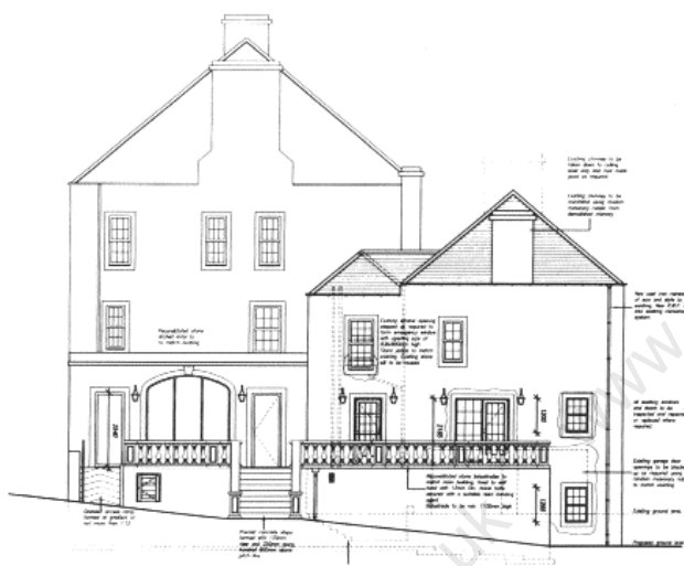
Gable end elevation of converted Victorian Wing (right) and new swimming pool (left) with main house behind.
